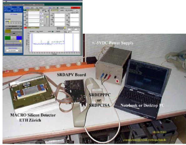
\*APV Readout Controller Software
