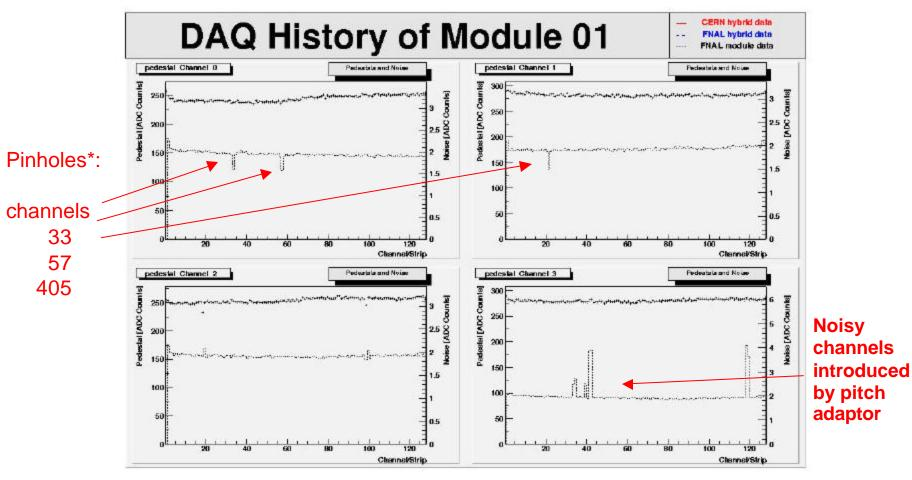
\*Channels disconnected from readout due to pinholes show lower noise
