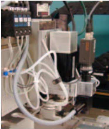
Figure 2: The bracket upon which the \phi motor, pick-up head and camera are mounted.
