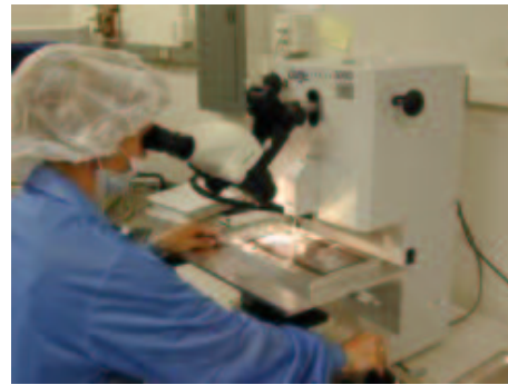
Figure 18: The DAGE model 3000 wirebond pull tester.
