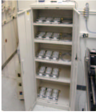
Figure 14: The cabinet used to store the modules during glue curing.
