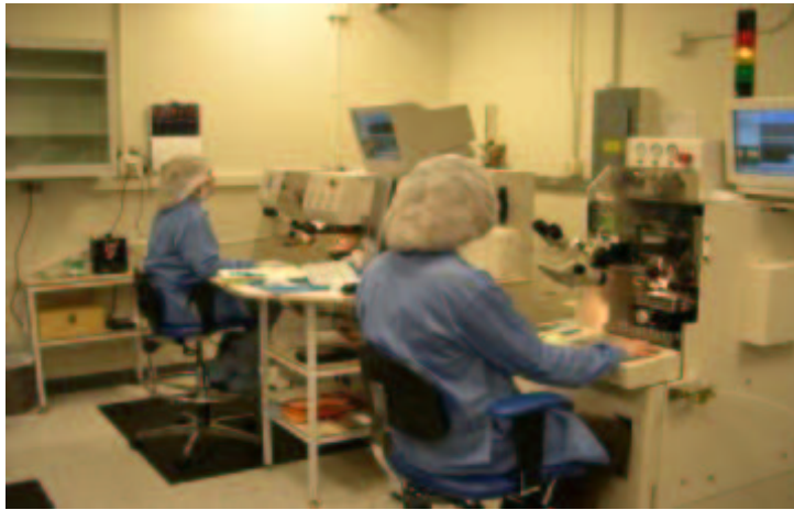
Figure 16: The K&S 8090 (left) and 8060 (right) wirebonders.
