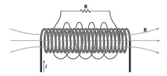
magnetic field points to the right. At time t=0 the solenoid current begins to decay exponentially as  $I_S(t)=I_0e^{-\frac{t}{\tau}}$ .
